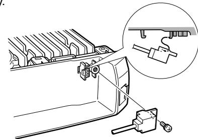
3 Connect the other end of the connectorized front panel cable to the One Touch panel.
