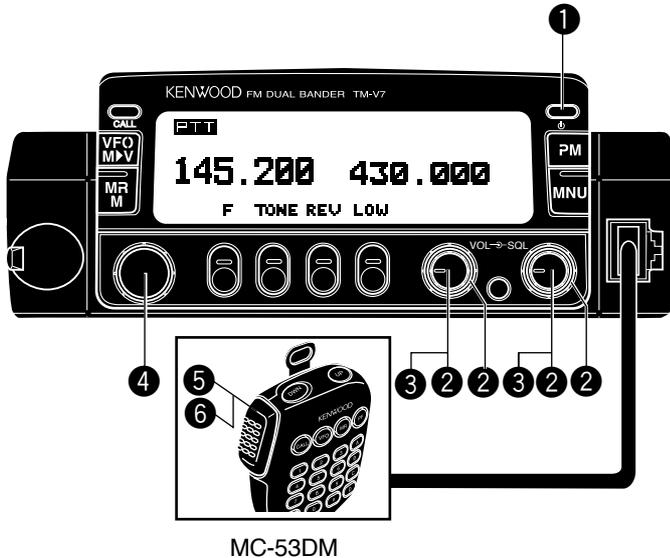
1 Switch ON the DC power supply, then press the  $\phi$  switch.
