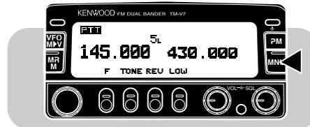
Lockout for an individual channel can be canceled by repeating the above procedure.
