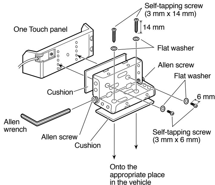
**Note:** Consider the safety of driver and passengers when deciding where to install the front panel. Tighten all screws firmly.
