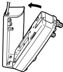
5 Assemble the mounting brackets, and install the front panel on the appropriate place in the vehicle.
