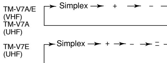
If the offset transmit frequency falls outside the allowable transmit frequency range, transmitting is inhibited until the transmit frequency is brought within the band limits by one of the following methods:
